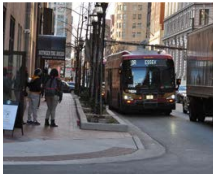
Travelway widths balance narrow lanes for speed control with safely accommodating the movement of transit and trucks.
